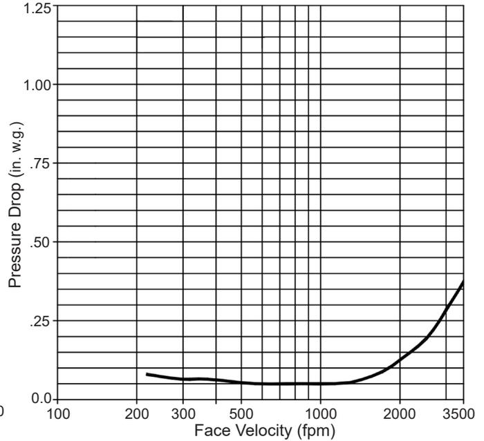
Typical performance for Model PC850 backdraft damper size tested 42"W x 42"H, furnished with counterweight to assist opening.
