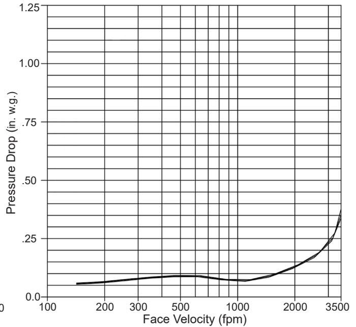
Typical performance for Model BIP9 backdraft damper size tested 42"W x 42"H furnished with counterweight to assist opening.
