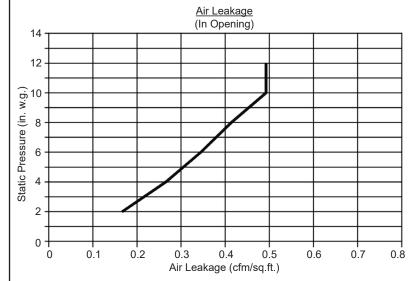
Air leakage chart is based upon independent air leakage tests conducted by Architectural Testing Laboratory. The out-opening model of a 24" x 60" AHF-T4I was tested. Tests were in accordance with ASTM E 283-91 "Determining the Rate of Air Leakage through Exterior Windows, Curtain Walls, and Door under Specified Pressure Differences Across the Specimen". Cesco Products recommends using out of opening doors for draw through applications and in opening (IO) for blow through applications.
