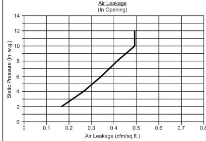
Air leakage chart is based upon independent air leakage tests conducted by Architectural Testing Laboratory. The out-opening model of a 26" x 60" AHF-T2I was tested. Tests were in accordance with ASTM E 283-91 "Determining the Rate of Air Leakage through Exterior Windows, Curtain Walls, and Door under Specified Pressure Differences Across the Specimen". Cesco Products recommends using out of opening doors for draw through applications and in opening (IO) for blow through applications.
